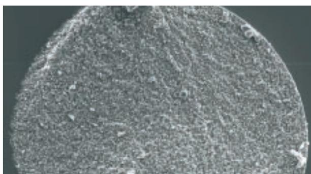
Figure 1 | FE-SEM picture of a cut through a Kromasil 300 Å particle at 5,000 × magnification.
