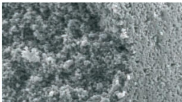
Figure 2 | FE-SEM picture of a cut through a Kromasil 300 Å particle at 35,000 × magnification, showing both the outer surface and the fracture through the particle.
